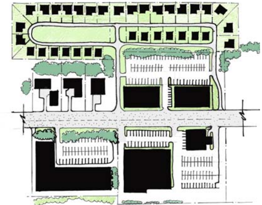
This proposal for the redevelopment/expansion of an existing commercial strip illustrates several important concepts: 1) parking is located to the rear of new retail establishments; 2) existing retail parking is set back from the roadway and is buffered by landscaping strips; 3) landscaping is used effectively to buffer parking/retail areas from existing residential uses; and 4) parking areas use shared entry/exits to the street thus minimizing curb cuts.
