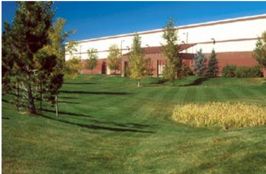
The rear of this "big box" store includes a generous landscaped buffer that also serves as a runoff detention basin for the parking areas
